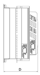
Control voltage (terminal A1, A2) = 230AC D = 147 Digital control voltage (terminal 1-5) = 24DC H = 245 Kg = 3.2 W = 122
